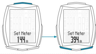
Setting by means of the sea level pressure.
