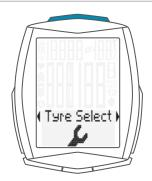
Press the **BIKE** or **TPC button** to scroll through the tyre list until your tyres are displayed (in the example shown  $29 \times 2.40$ )
