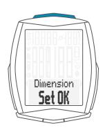
You can set the roll circumference of your wheel in millimetres on the VDO M6 or select the applicable tyres from a tyres table.
