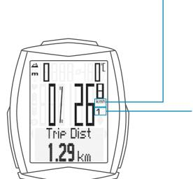
On the right of the display, under the speed indicator, the unit kmh or mph is displayed.
