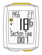
Press the **BIKE button** to scroll to the trip section.
