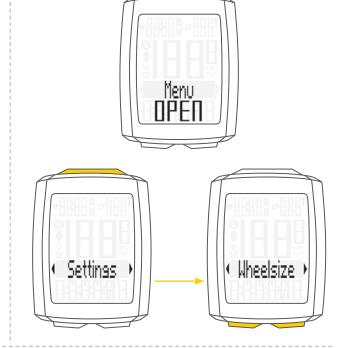
Press the **SET button** to open the setting for the **wheel size**.
