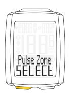
Based on the calculated or set HR max, the calculated or set lower and upper limits for the respective training zone will appear on the display.
