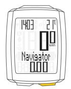
Once the navigator function is on the display, press and hold the SET button until the settings menu opens.
