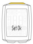
You can set the roll circumference of your wheel in millimetres on the VDO M5 or select the applicable tyres from a tyre table.
