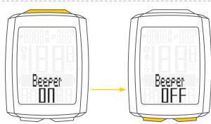
Press the **SET button** to confirm the setting. The response **"Set OK"** appears on the display.
