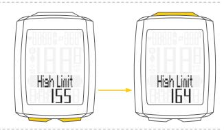
Press the **SET button** to confirm the value you have set. The response **"Set OK"** appears on the display.
