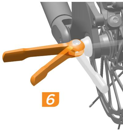
Clamping force is sufficient if the lever leaves an imprint on your hand and the adjusting nut is engaged with at least 4 threads on the axle. To increase clamping force, open the lever and turn the adjusting nut clockwise. Close the lever to recheck clamping force. Repeat until the clamping force is sufficient, then close the lever. If further attempts to center align the wheel fail, consult a professional bicycle mechanic.
