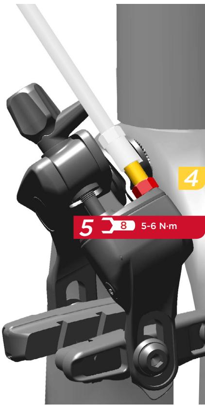
Install the hose firmly into the brake caliper while threading the compression nut by hand. While holding the hose firmly in place, use an 8 mm flare nut wrench to tighten the compression nut to 5-6 N·m (44-52 in-lb).
