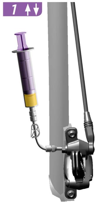
Hold the syringe at the caliper vertically. Firmly pull on the plunger to create a vacuum, then compress the plunger to pressurize the system. Repeat this process several times or until only a small amount of bubbles exit the system.
