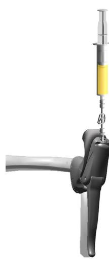
Hold the caliper syringe vertically. Gently push the caliper plunger down, stopping when the caliper syringe is 1/4 full and the lever syringe is 1/2 full.
