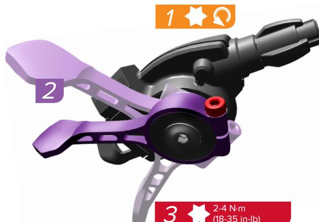
Loosen the reach adjust bolt to adjust the shift paddle to the desired angle, then tighten the bolt to 2-4 N·m (177-3.4 in-lb).
