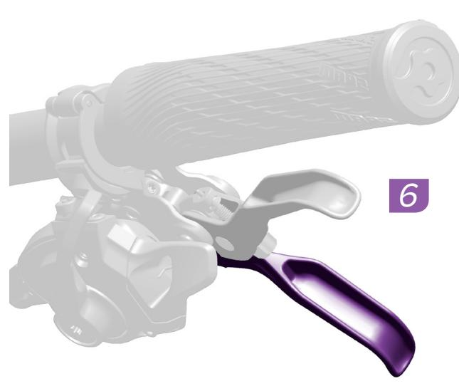
Pull the brake lever to the handlebar, tighten the caliper bolts to 9-10 N·m (80-90 in-lbs), then release the brake lever.
