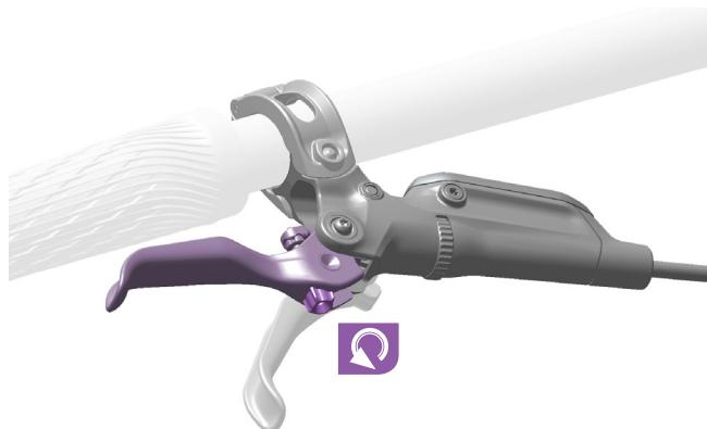
Turn the reach adjust counter-clockwise to move the lever blade closer to the handlebar.
